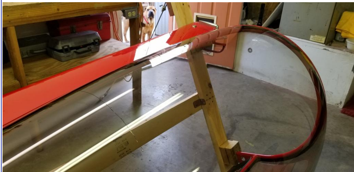
A Dremel #125 V-groove bit was used to begin the process of opening up the crack channel and relieving some of the built-in stress on the acrylic.
