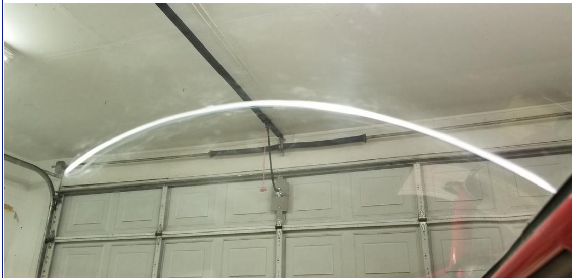
The surgical area was once again cleaned with solvent then prepared from inside the canopy using aluminum tape. The tape served a double function of stabilizing the plexiglass, freeing up any distortion while preventing the bonding material from dripping through.
