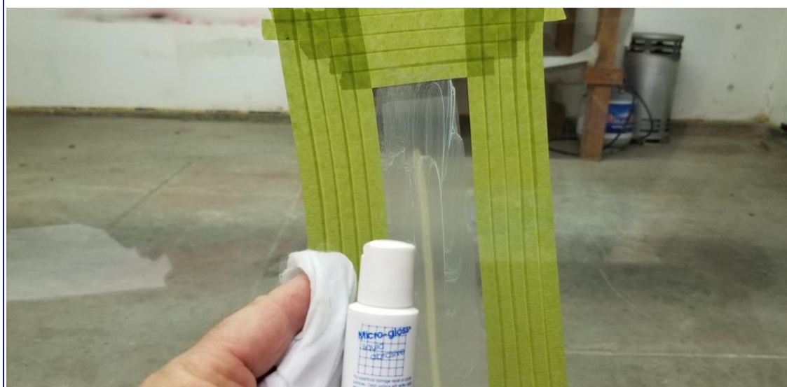
The canopy orientation was again reversed to complete the polishing stages on the exterior surface.
