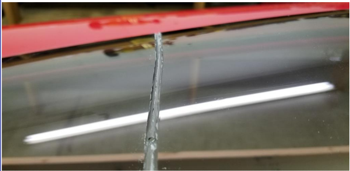
The crackline was clearly visible as the V-groove deepened.
