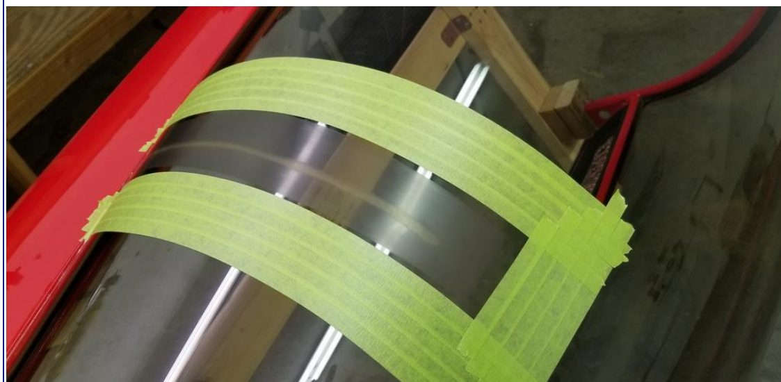
The canopy orientation was again reversed to complete the polishing stages on the exterior surface.
